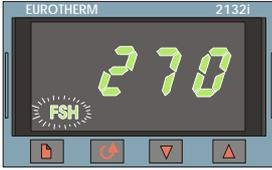
The Eurotherm 2132i over-temperature limit controller monitors the furnace chamber temperature using an independent measurement circuit. If the furnace chamber temperature rises above the configured value (generally  $T_{max} + 30^{\circ}\text{C}/86^{\circ}\text{F}$ ), the heater is turned off by a safety fuse to protect the furnace – "FSH" alarm flashes on the over-temperature limit controller.
